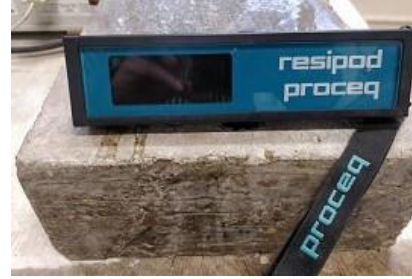
Fig. 3 – Electrical Resistivity using four point wenner probe technique
