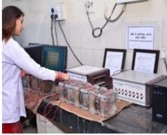
Fig. 2 – Rapid chloride Penetration test (RCPT)
